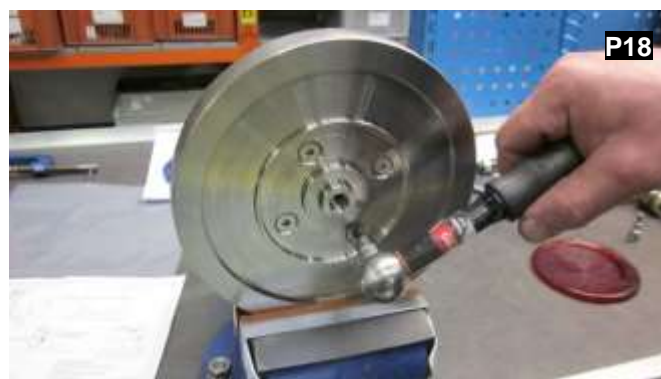
Grip the pressure plate in a soft jaws vice and loosen the bolts using a 5/32" torque wrench.
