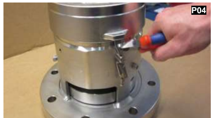
Cut the TIR wire and remove it by feeding it through the cable nipple.
