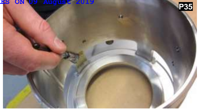
Apply Rocol on the 4 segments of the body tube. Lubricating assists smooth movement of the pressure plate.
