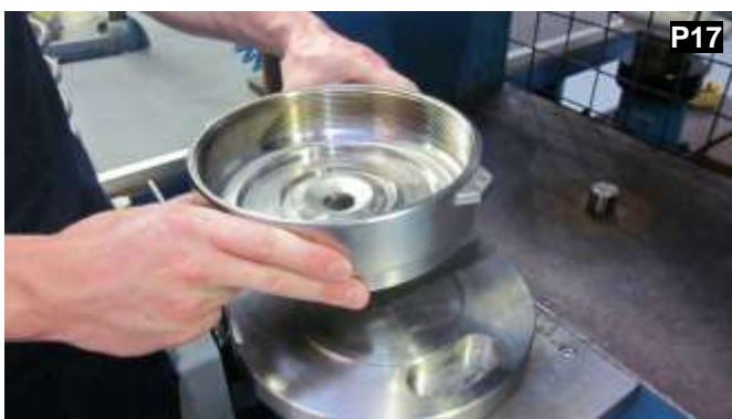
Remove the top cap. Inspect the top cap for any damage.
