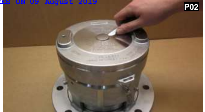
Use a sharp edged tool to detach the stainless steel plug.
