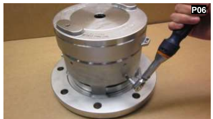
Use a 1/4" torque wrench or Allen key and loosen the three lift stops and remove.
