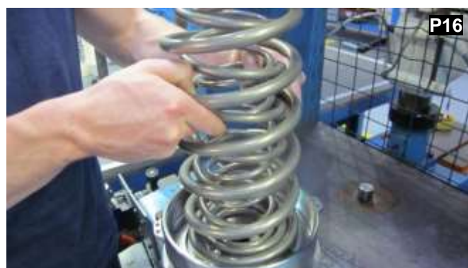
Remove the spring. Inspect the spring for any damage.
