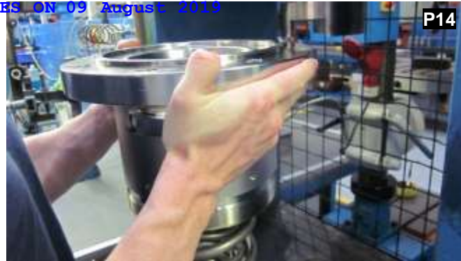
Once the spring is fully extended retract the ram completely allowing full access to the valve. Remove the main body. Inspect the main body for any damage.
