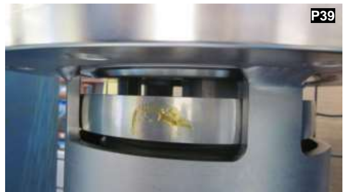
Continue lowering the ram until it has pushed the pressure plate free from the seal face, allowing the body to be lowered and screwed in to the cap. Ensure this gap exists throughout the entire circumference to avoid damaging the pressure plate o ring.
