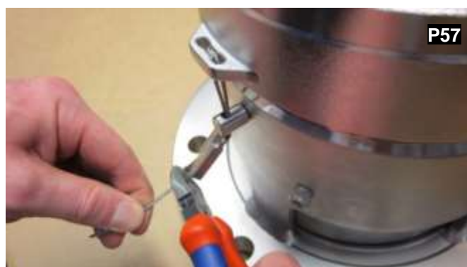
Cut the wire after ensuring that the remainder of the wire is pulled enough to make the loop tight.
