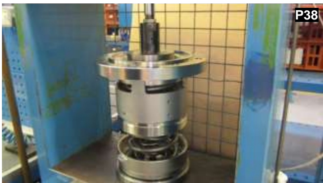
Bring the ram down ensuring not to touch the bore.
