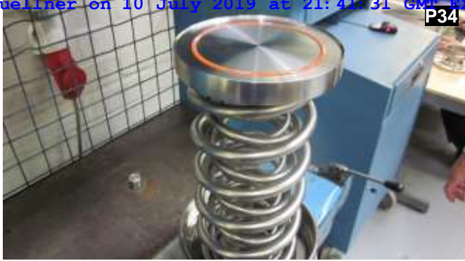
Locate the pressure plate assembly on top of the spring. Ensure the pressure plate groove is located in the spring.
