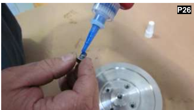
Apply blue Loctite 243 on the bolts. Locate and nip the bolts using a 5/32" torque wrench in a diametrically opposite sequence.
