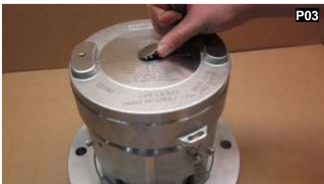
Remove the stainless steel plug.
