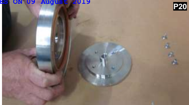
Remove the inner pressure plate from the outer.
