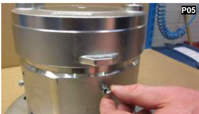
Remove the cable nipple.
