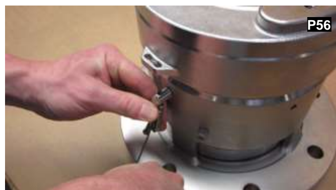
Feed the wire back into the gripper lock.
