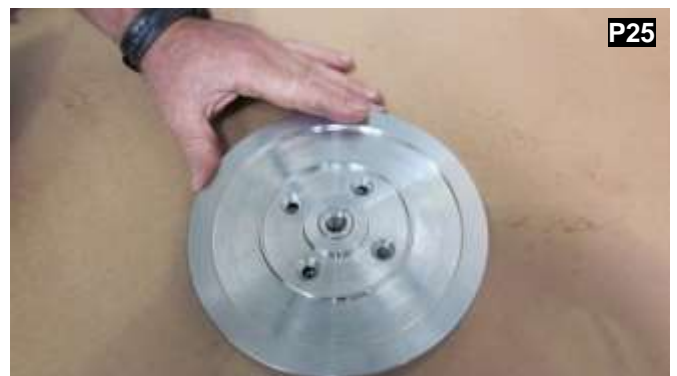
Align the holes in the outer pressure plate with the holes in the inner pressure plate.
