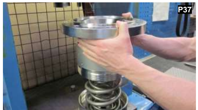
Slide the assembly towards the location pin on the press bed. Push the cap locator forward aligning the groove and the locating pin on the bottom of the press. This locates the assembly in the centre of the press and improves the alignment of the ram and the bore. Please refer P29.
