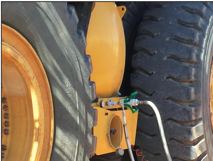
LNG fueling application on off-highway mining truck
