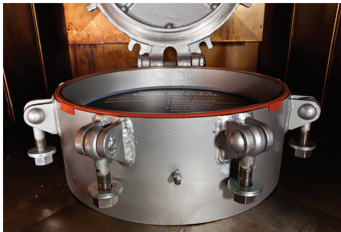
Figure 1: Alignment tabs (4) located on outside of manway nozzle.
