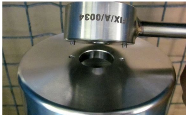
Step 38. Select the cap tightening tool, part number FIX/A/0034. Locate the two pins on the cap tightening tool into the two blind holes of the top cap.
