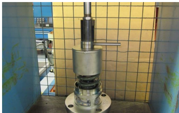
Step 12. When the valve and the cap are disassembled, unlock the press and gradually retract the press to release the spring load. WARNING: Be careful when you retract the press. Make sure that the spring is fully decompressed before you remove the ram.
