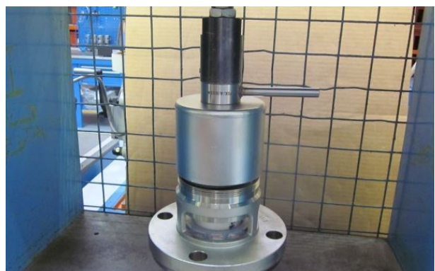
Step 40. Apply pressure slowly onto the top cap to compress the spring. CAUTION: Align the body with the cap to prevent cross-threading.
