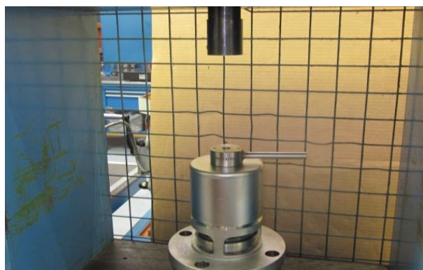
Step 10. Make sure that the cap tightening tool is installed correctly on the top cap.
