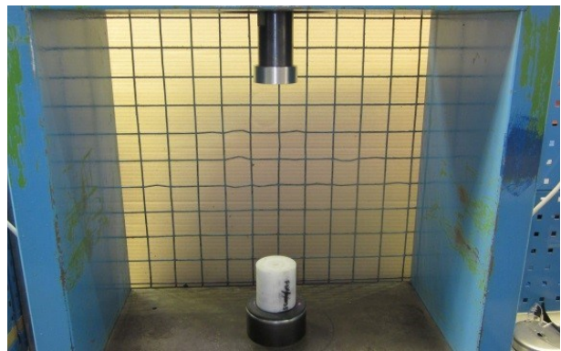
Step 36. Make sure that the top ram is retracted to allow enough space to accept the valve height.
