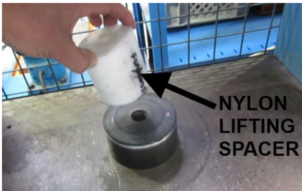
Step 35. Select the nylon lifting spacer, part number FIX/A/0035, and install it onto the bench press.
