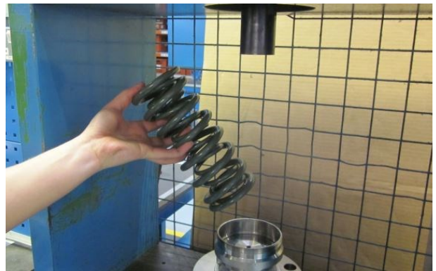
Step 16. Remove the springs. Examine the springs for signs of corrosion or damage. If there is damage, contact Fort Vale.
