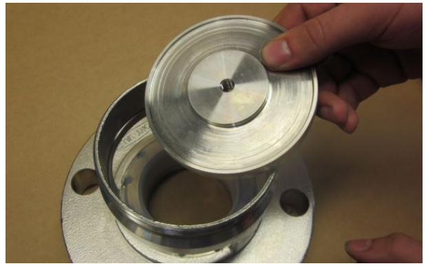
Step 20. Remove the pressure plate.
