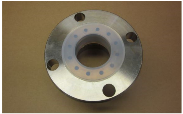
Step 22. Examine the PFA lined Super Maxi body for signs of damage. Look carefully at the pressure plate sealing face and the gasket sealing face. If there is damage, contact Fort Vale. The disassembly procedure is complete.
