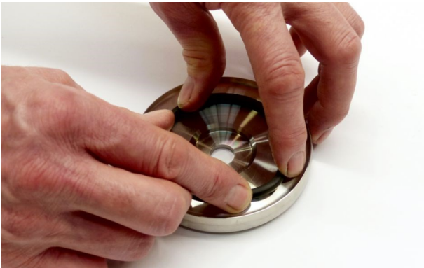
Step 86. Install the O ring into the outer pressure plate. Push the O ring around the circumference to install it into the groove.
