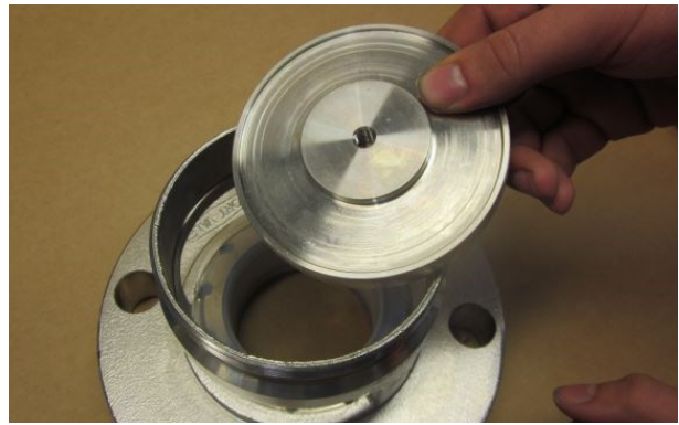
Step 20. Remove the pressure plate and identify the type.
