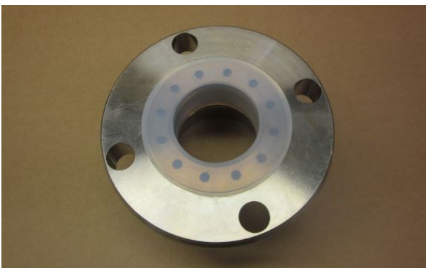
Step 23. Examine the PFA lined valve body for signs of damage. Look carefully at the pressure plate sealing face and the gasket sealing face. If there is damage, contact Fort Vale. The disassembly procedure is complete.
