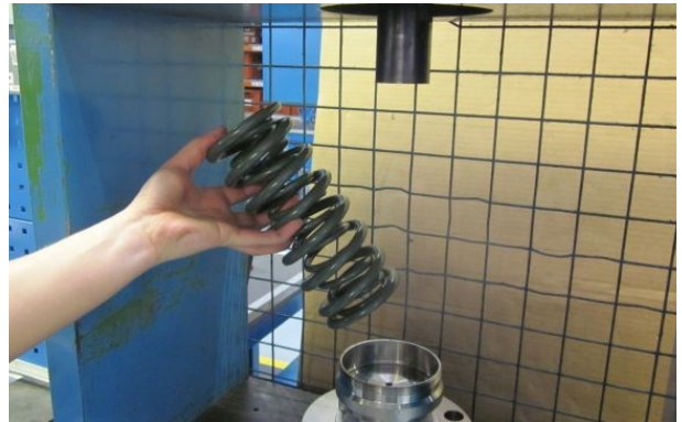
Step 16. Remove the springs and discard them.
