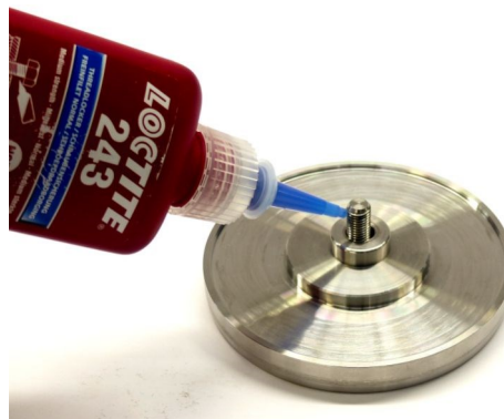
Step 89. Install the retaining washer. Apply thread adhesive to the thread of the stud.
