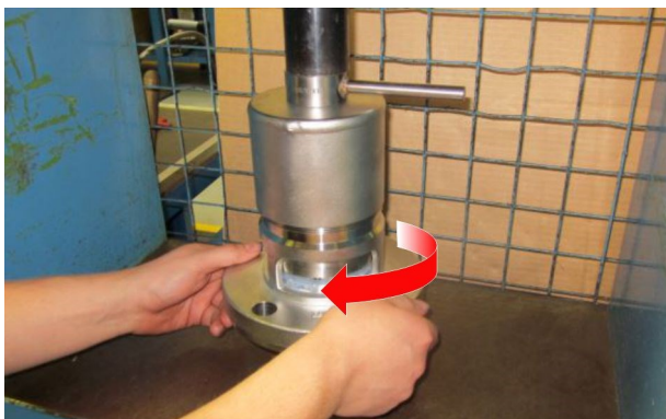
Step 11. Apply pressure onto the top cap tightening tool until the spring is compressed sufficiently so that the valve body is free to turn. Then turn the valve body clockwise until it is disassembled from the top cap. WARNING: Make sure that you lock the press before you start to unscrew the valve.
