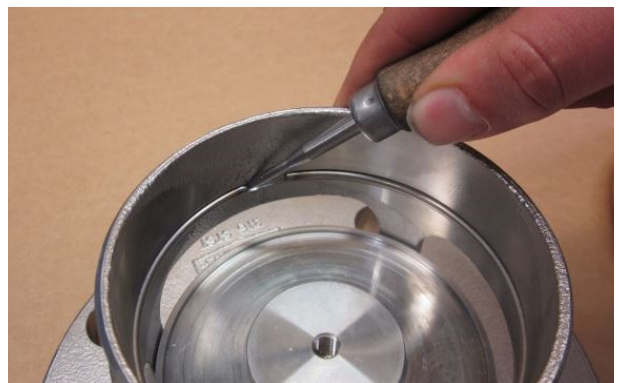
Step 18. Use a sharp-edged tool to detach the retaining ring clip. If the valve does not have a ring clip, go to Step 20.
