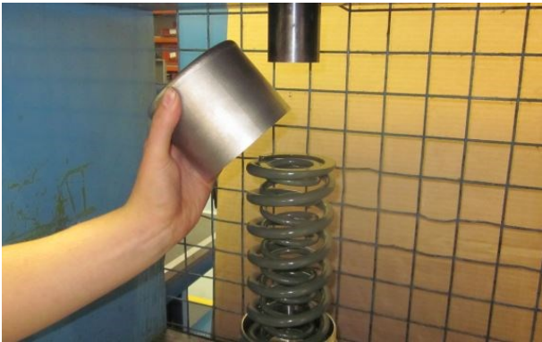
Step 15. Remove the top cap and discard it.
