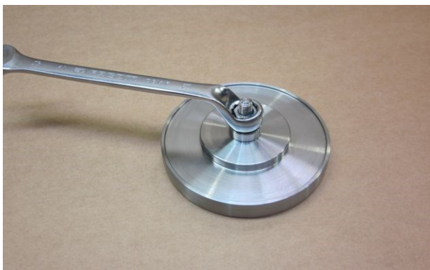
Step 94. REPLACE THE STUD: Use a 1/2" (13mm) spanner to loosen the 5/16" UNF nut on the pressure plate assembly.
