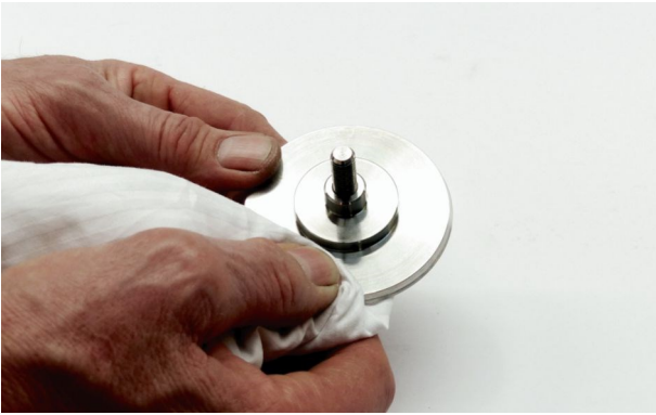
Step 84. Clean the inner pressure plate. Examine it for damage. If there is any damage, contact Fort Vale.
